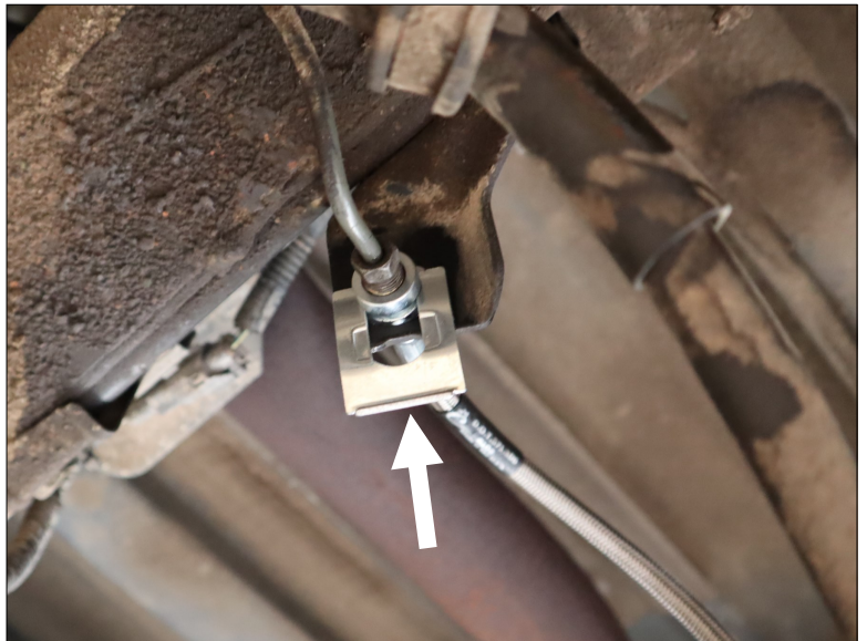
Replace clips where required. (Step 05)
