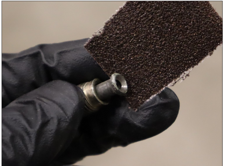
Sand the flare if required. (Note C)
