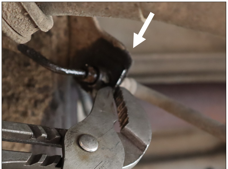
Remove clips if present. (Step 03)
