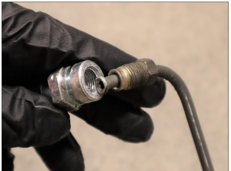
Compare the flare to the threaded internal diameter. (Note B)
