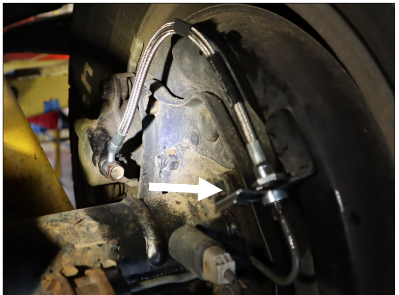
Rear shown: Torque the bolt and secure line with a clip. (Step 09)
