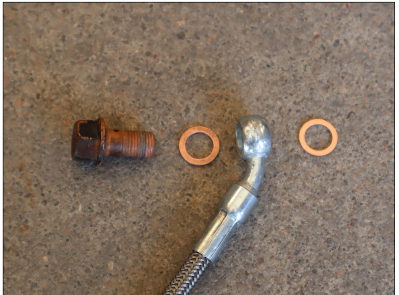
Use new washers with the banjo bolt. (Step 08)
