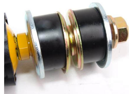
Washer, bushing and nut orientation (Step 6)
