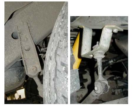
Photos showing the two different swaybar mounts that were used on the '91-'97 Land Cruiser
