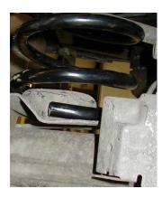
Rear spring installed and end of coil seated properly.
