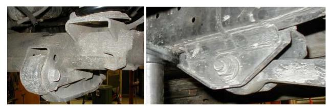
Front control arm mounting bolts. These bolts are removed by loosening the bolt and not the nut. The nuts have serrations on the face and it locks in place.
