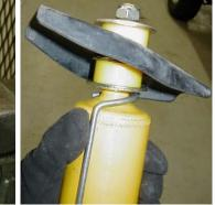
Removing shock from mounting plate
