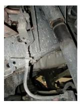
Passenger side brake line bolts removed.
