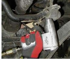
Removing the front swaybar bracket bolts.
