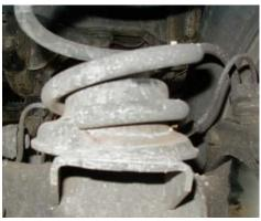
Driver side spring unloaded. Not the position of the end of the coil. Make sure the new springs are installed with the end of the coils in the proper location.
