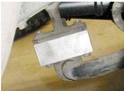
Swaybar block installed on front swaybar.
