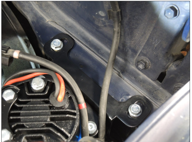
Install compressor and bracket in vehicle (Step 8)
