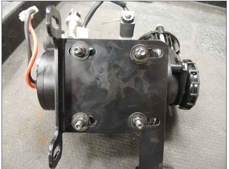
Mount compressor to bracket (Step 7)
