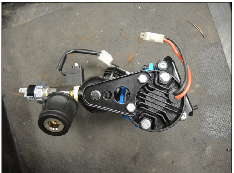
Orient fittings and compressor in sleeve as shown (Step 6)
