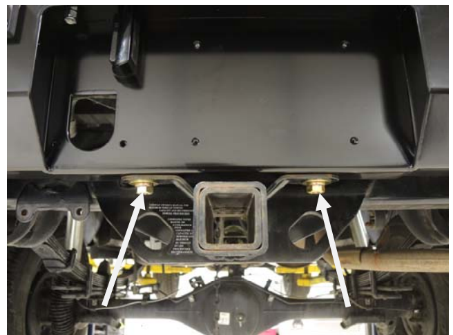
Receiver installed with bumper detail ( step 6D )
