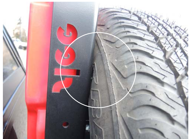
Adjust tire mount to set proper preload (step 16B)
