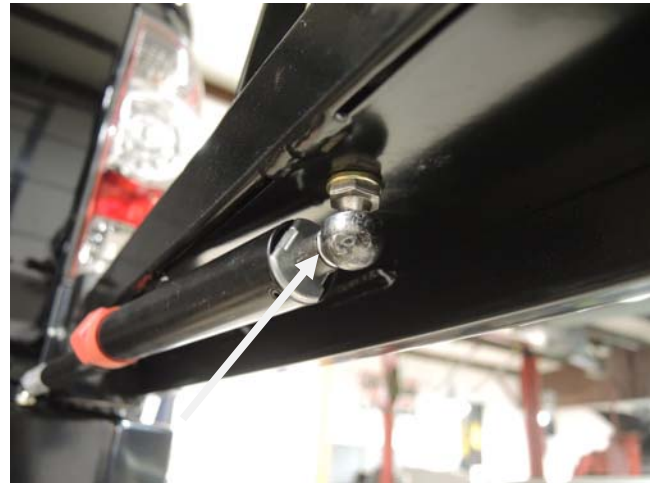
Install Carrier shock (step 15)
