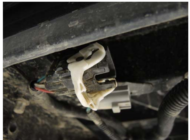
Disconnect and remove harness (step 1A)
