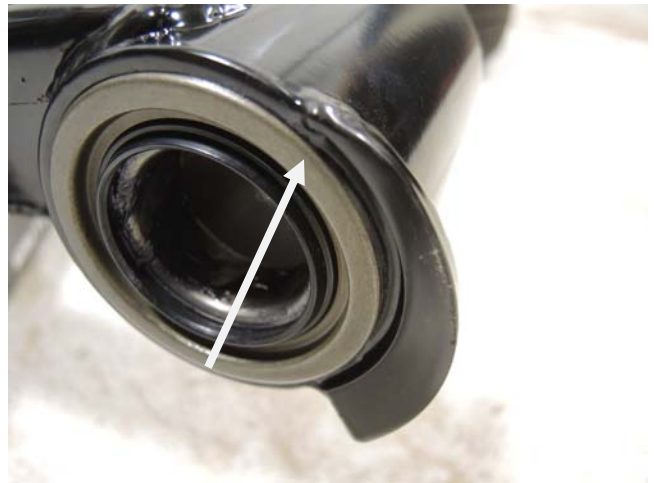
Install hub seal (step 13A)
