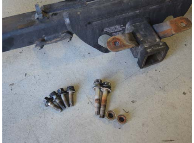
Separate receiver from bumper (step 2D)
