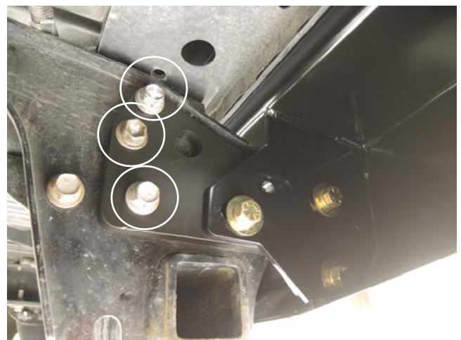
Driver side Frame Bracket detail (step 6A)
