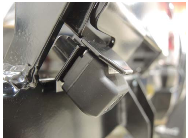
Install Camera to Slee Bracket (step 18B)
