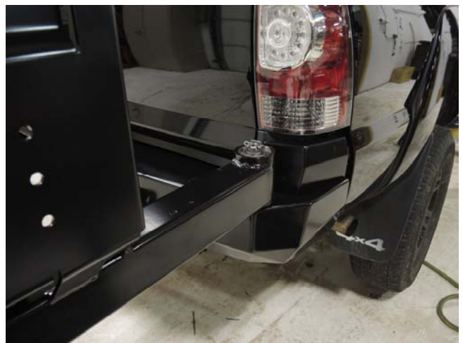
Install Carrier on Spindle (step 14C)
