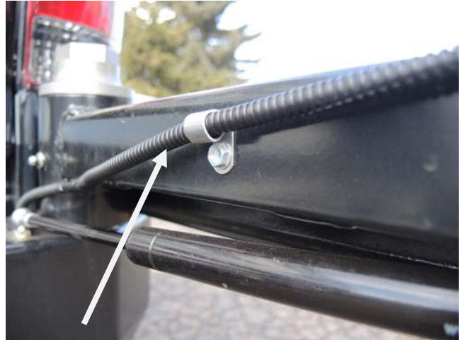
Secure camera harness with supplied clip and screw ( step 18C )
