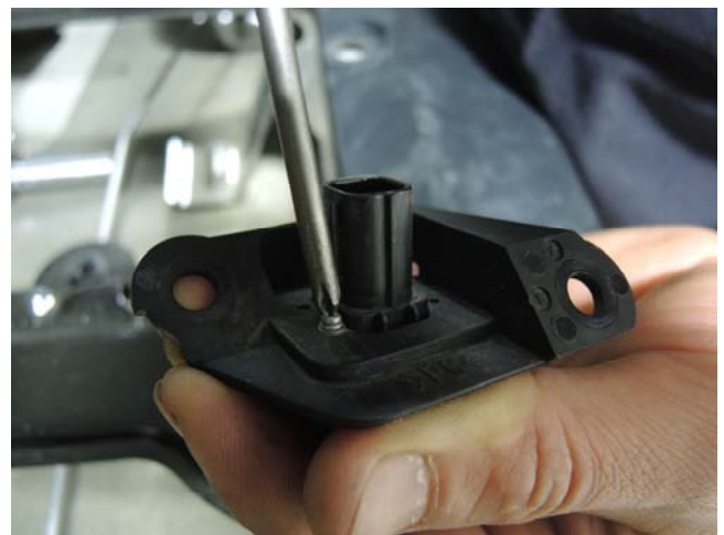
Remove Camera from bracket (step 17C)
