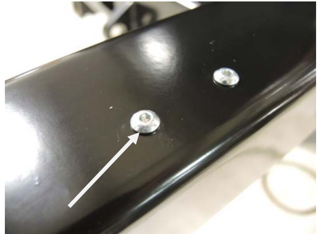
Install Hi-Lift Bracket, if not used install two 10-32 screws into swing arm ( step 23 )
