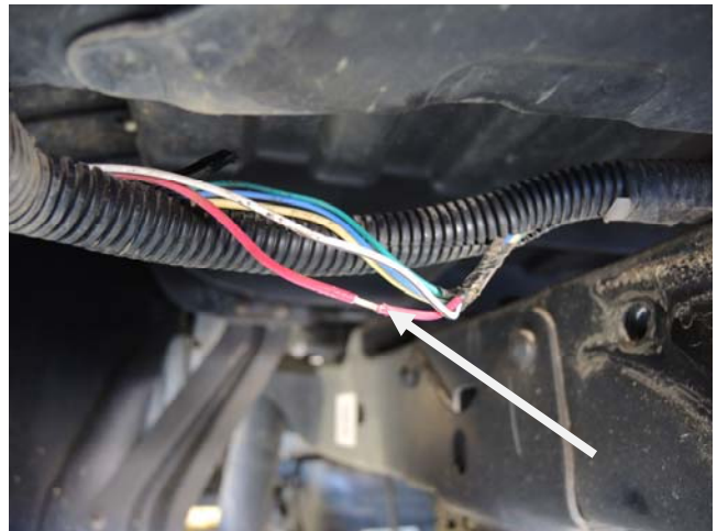
LED Light reverse trigger location (step 10B)
