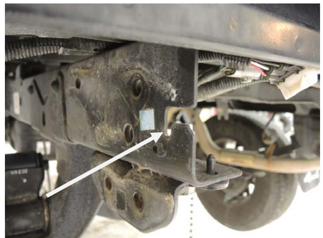
Locating tab frame side shown (step 2C)
