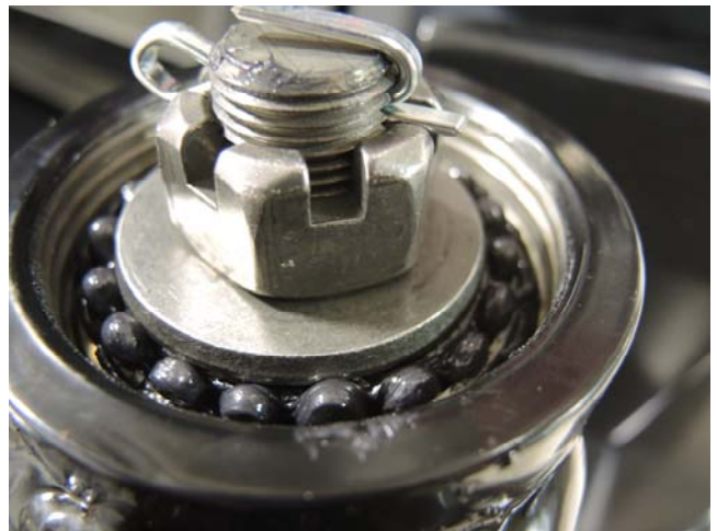
Install Carrier on Spindle (step 14B)
