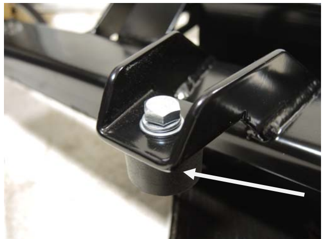
Install Rubber Bump Stop (step 13B)
