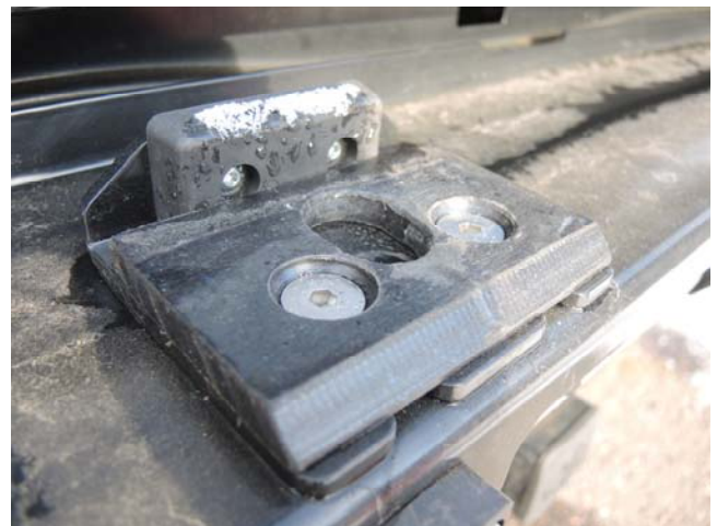
Assemble and install Nylon Pad with Bracket (step 5)
