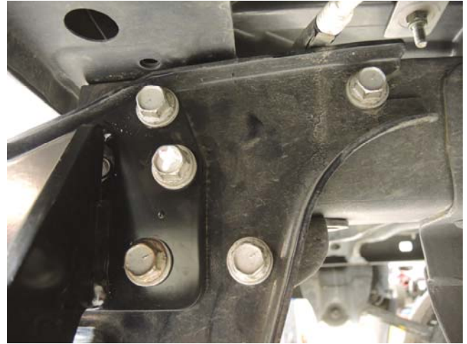
Passenger side Frame Bracket detail ( step 6B )
