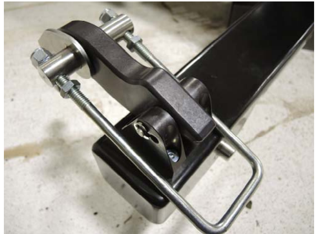
Pre-assembled Slee latch (step 14A)
