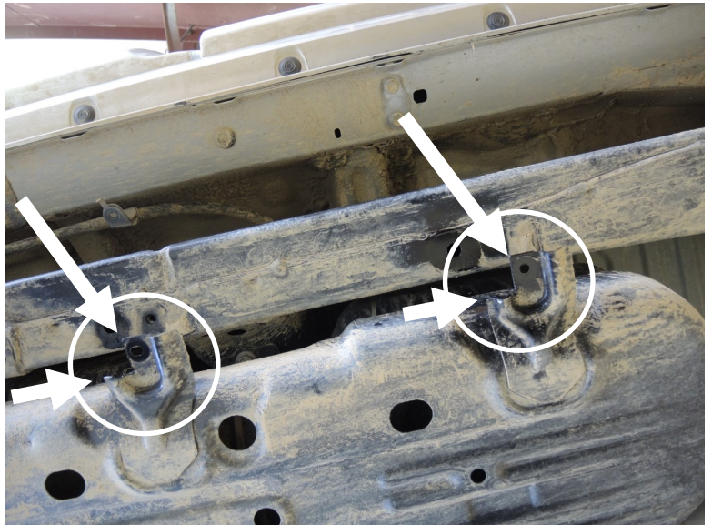
Trim the fuel tank brackets as shown. (Step 4)
