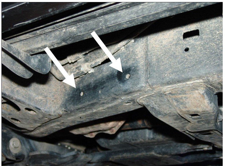
Install M8 rivet nuts into the driver side frame rail (Step 6).
