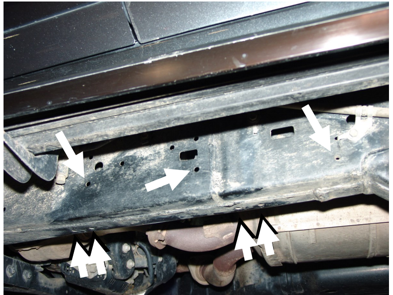
Install M8 rivet nuts into the driver side frame rail (Step 7).
