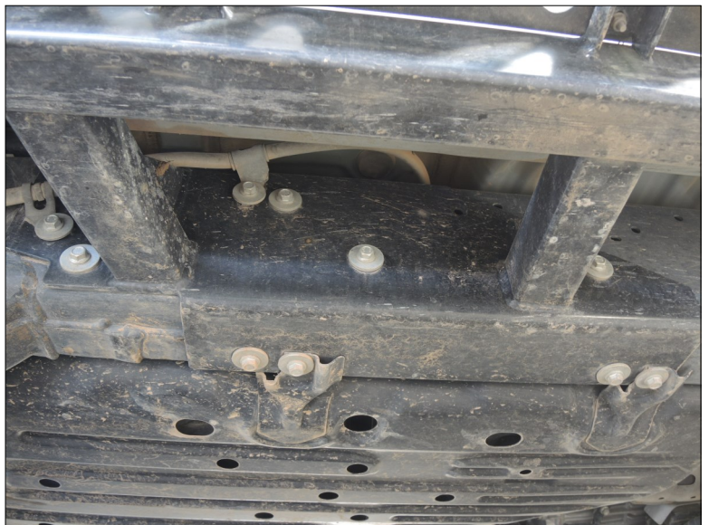
Rear passenger leg with fuel tank skid installed. (Step 13)
