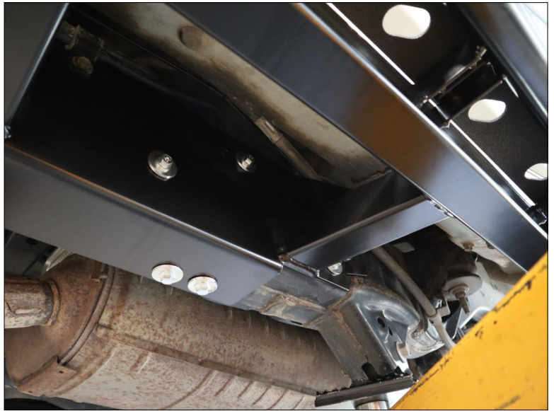
Rear driver leg installed. (Step 8)
