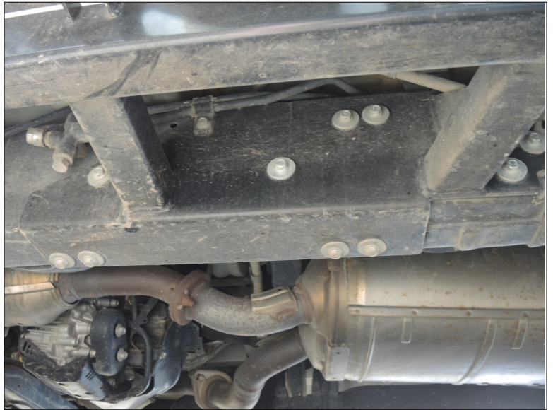
Rear driver leg installed. (Step 10)
