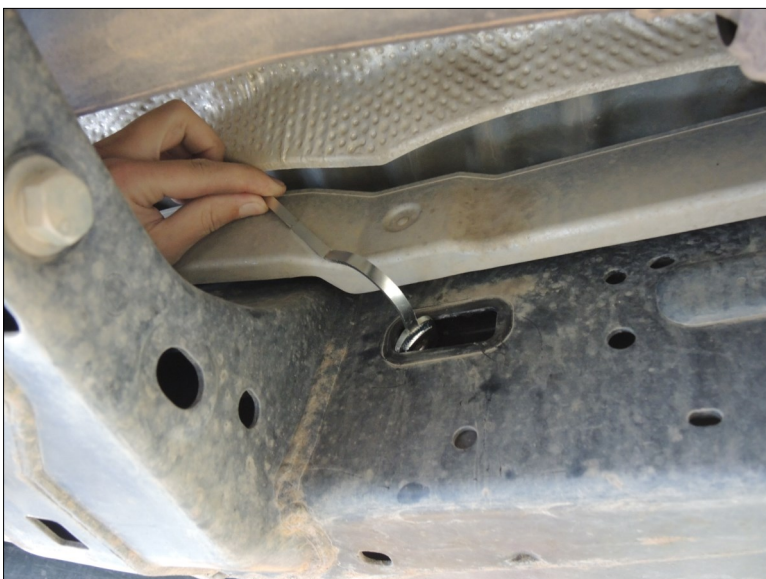
Remove the plug and place the nut inside the frame rail. (Step 9)
