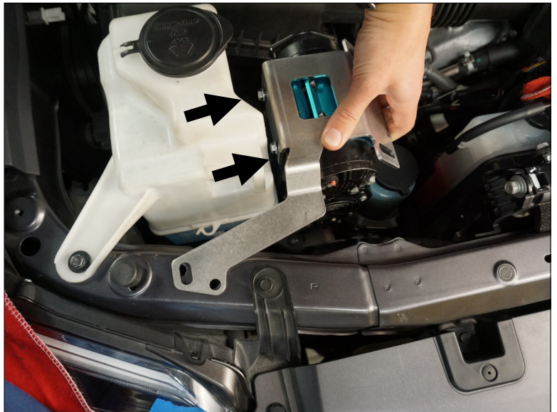
Install the upper bracket. (Step 11)
