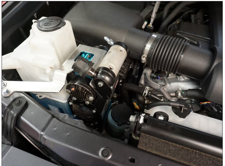
Attach the manifold to the upper bracket. (Step 13)
