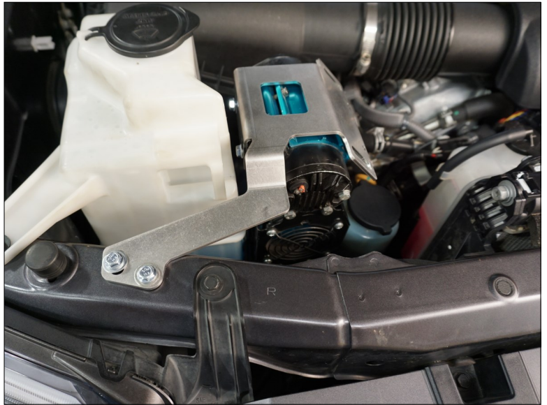
Install the nut plate. (Step 12)
