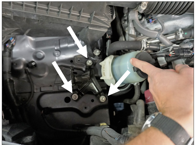
Remove the power steering reservoir bracket. (Step 3)
