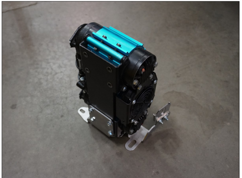
Attach the ARB twin to the lower bracket. (Step 8)
