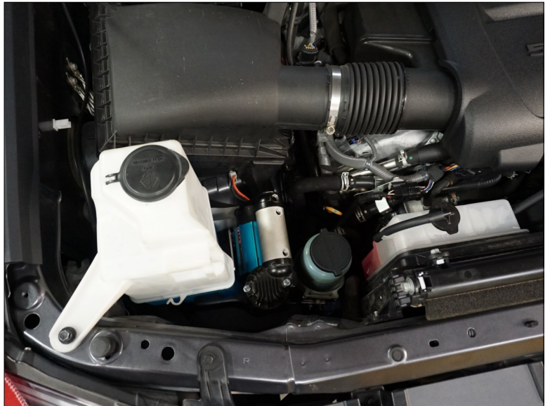
Reinstall the washer reservoir. (Step 7)
