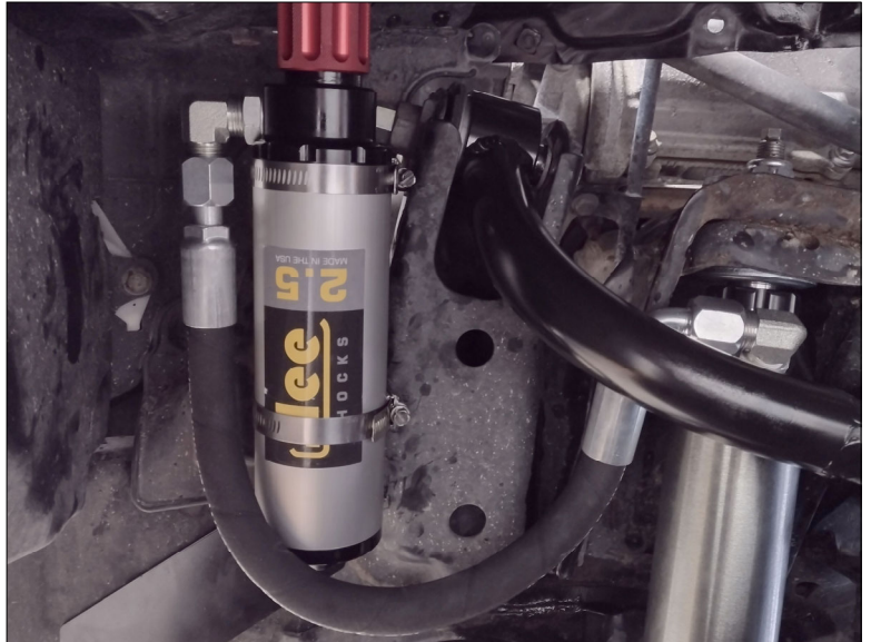
Hose and reservoir mounting for clicker reservoir—Driver Side. (Step 6)
