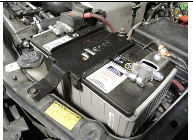
Install battery and tie down bracket (Step 6)
