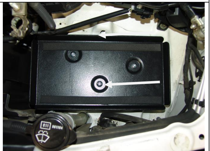
Install Adhesive Pads ( Step 4A )
