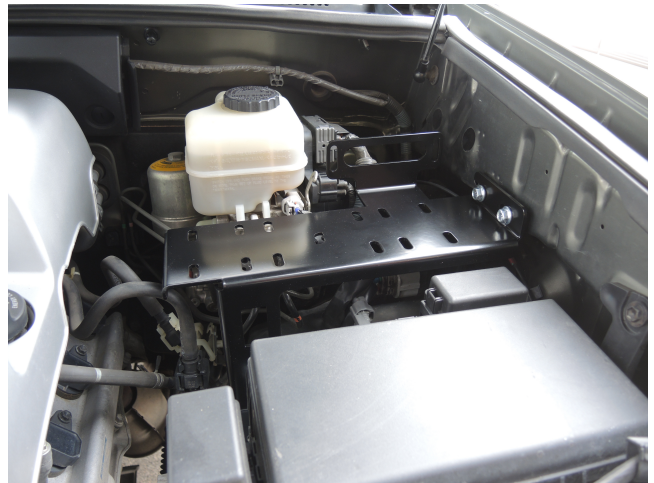
2003-2009 Lexus GX470 installation complete (step 5C)
