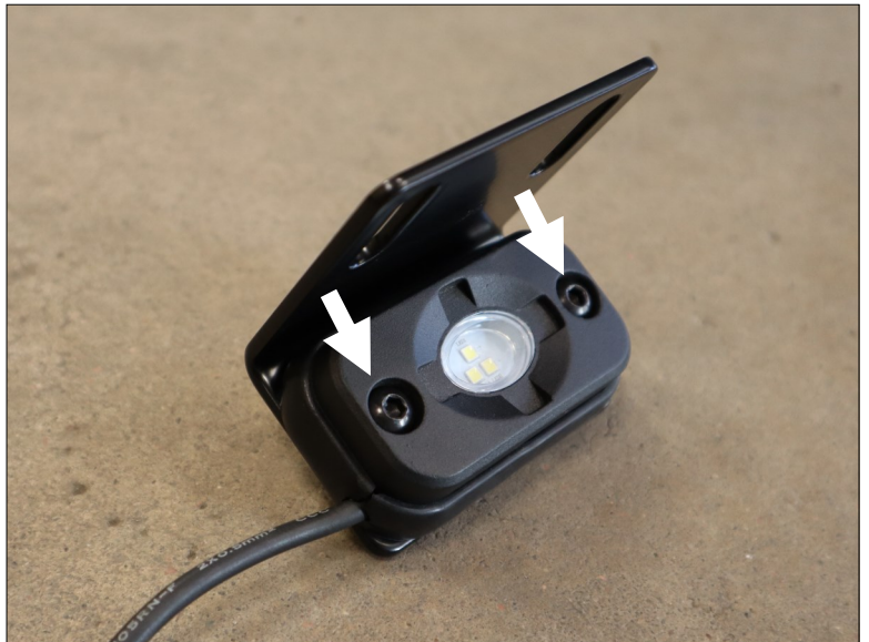
Attach the LED to the bracket. (Step 2)
