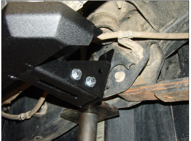
Mount the rear leg bracket. (Step 9)
