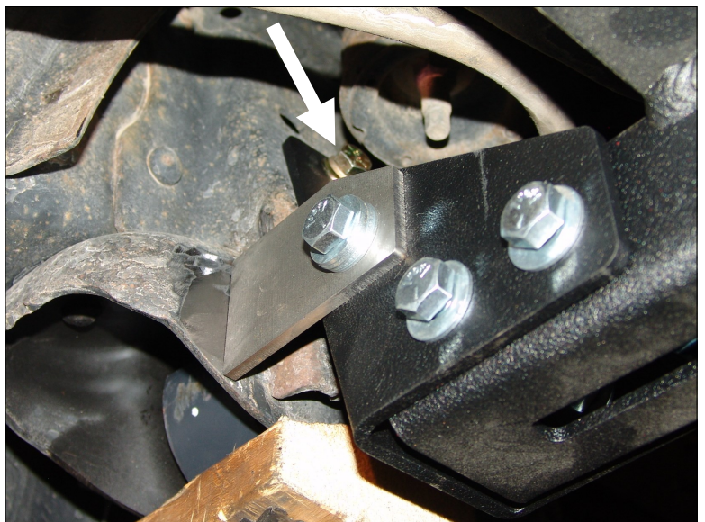
Bolt the leg bracket to the frame. (Step 9)
