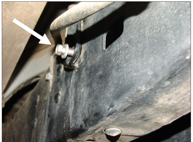
Remove the wire harness bracket. (Step 3)
