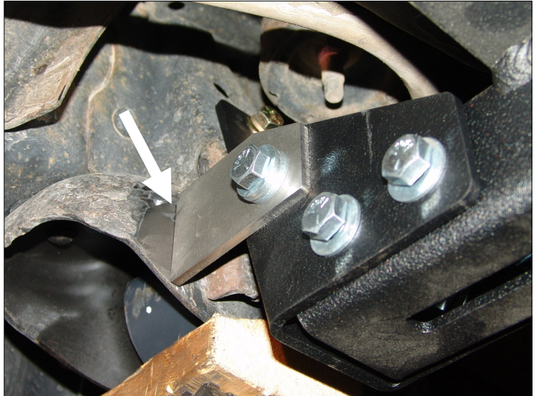
Bolt the leg bracket to the frame. (Step 10)
