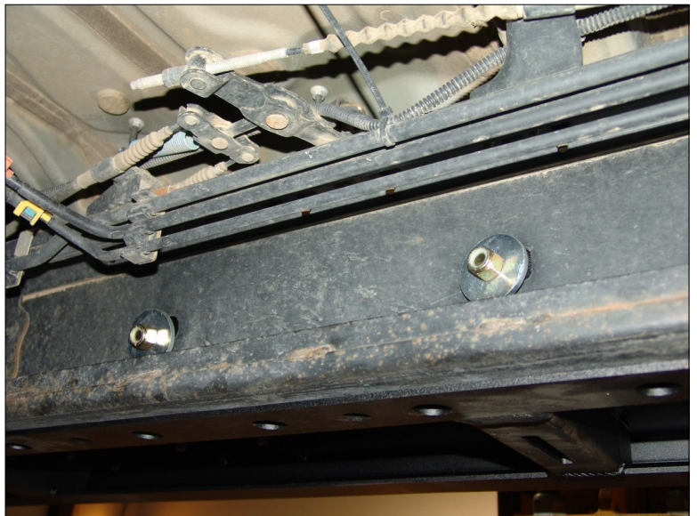
Bolt the slider to the frame using thick washers. (Step 7)
