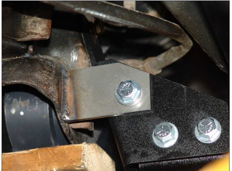
Weld the tab to the frame. (Step 11)
