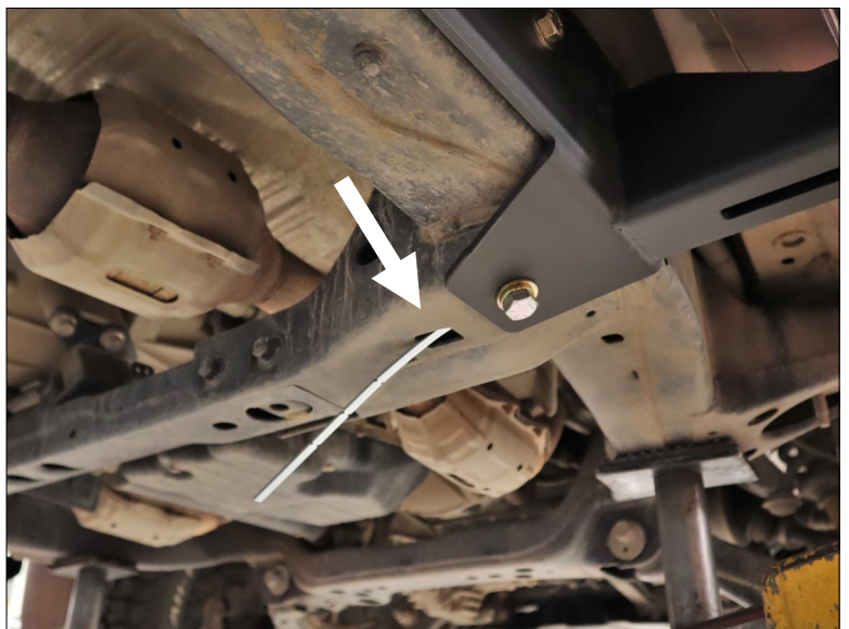
Install the hardware through the frame. (Step 8)
