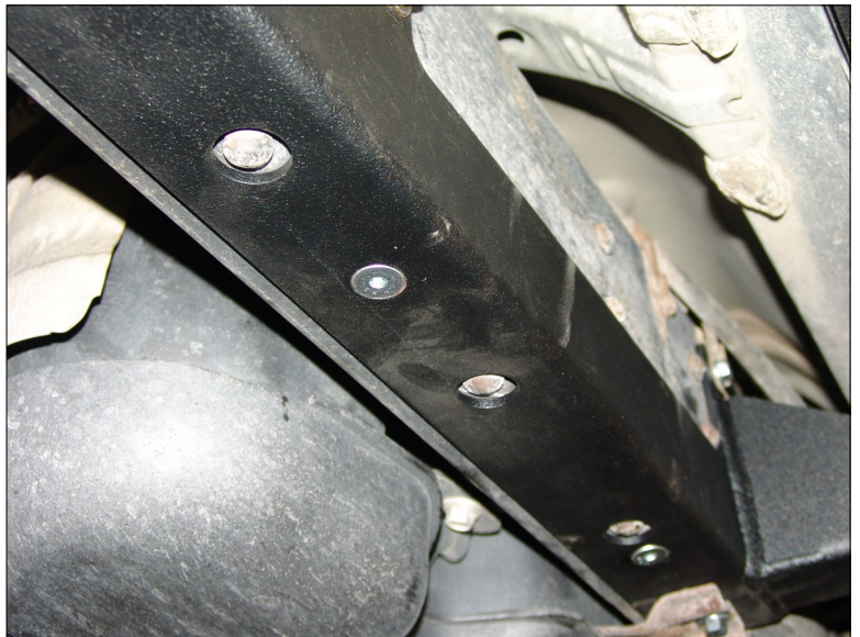
Install the lower hardware. (Step 13)
