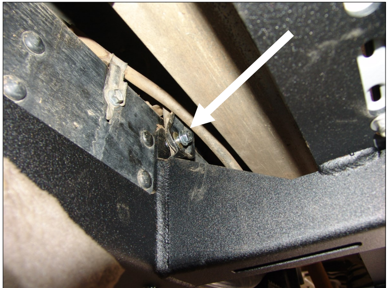
Reinstall the harness bracket. (Step 5)
