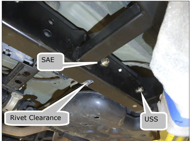
Install the driver side slider. (Step 10)
