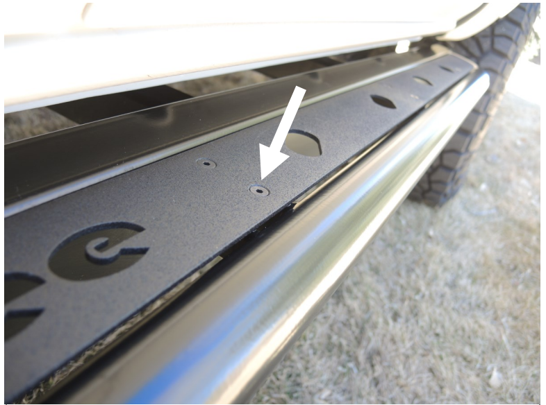
Install the SliderStep inserts. (Step 1)
