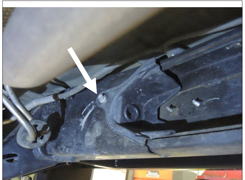
Inside frame view: Remove the frame rail cap if equipped. (Step 4)
