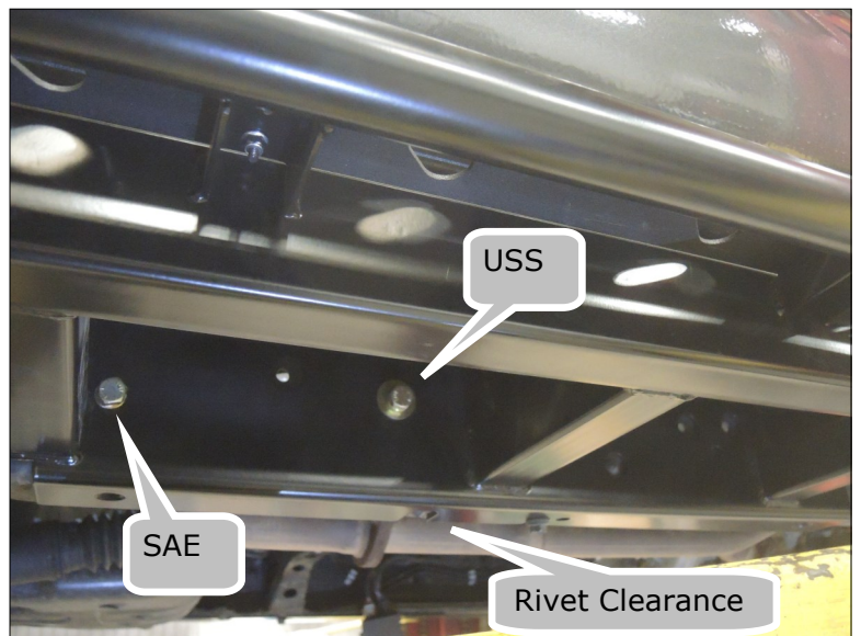
Use 3 bolts to keep the passenger slider in place. (Step 3)
