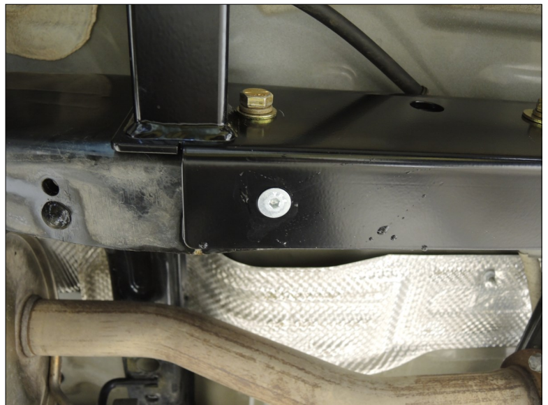
Install the countersink bolts on the underside of the slider. (Step 6)
