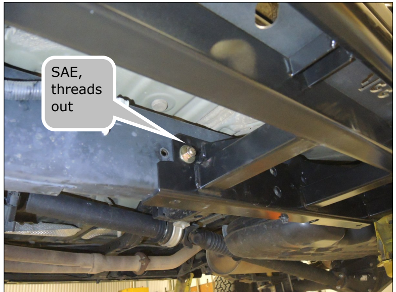
Install the forward bolt with the head inside the rails. (Step 11)
