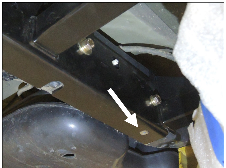
Drill the holes under the slider rail. Install the hardware.(Step 13/14)
