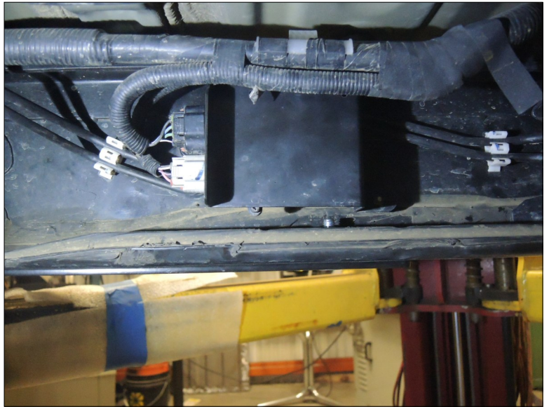
Reinstall the relay box. (Step 15)
