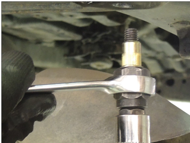
Step 2: Prep for Rivnut installation
