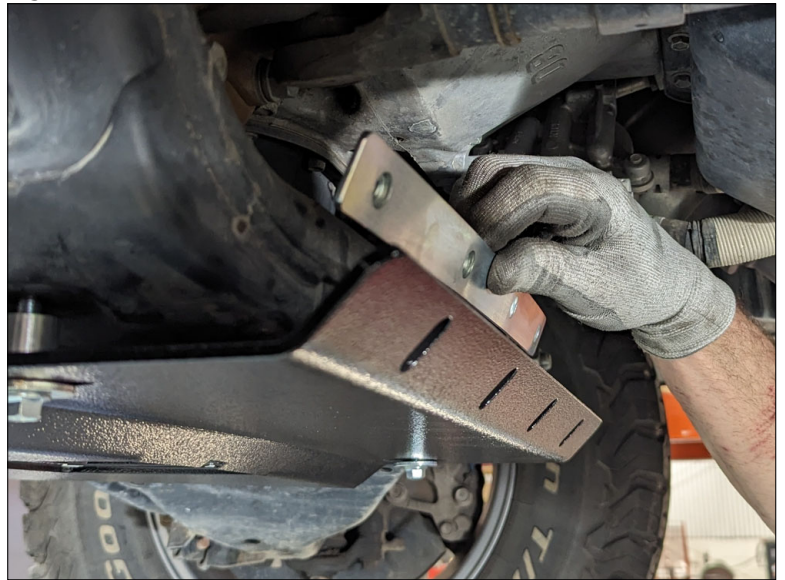
Step 4: Insert nut plate
