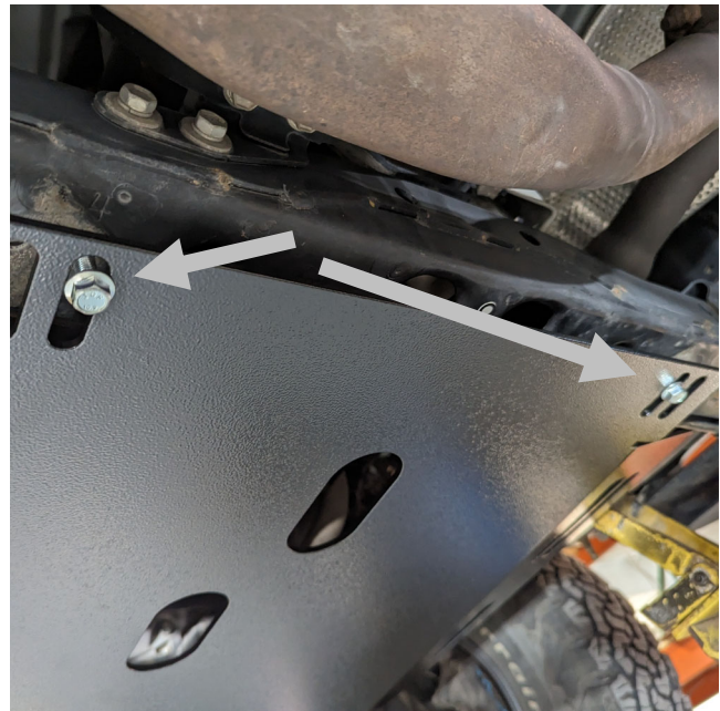
Step 4: M8 Flange bolts installed in innermost slots.
