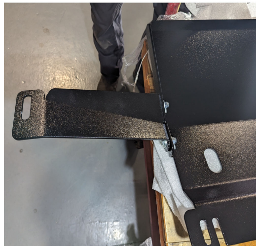
Step 5: Transfer Case Bracket installed on Transfer Case Skid Plate.
