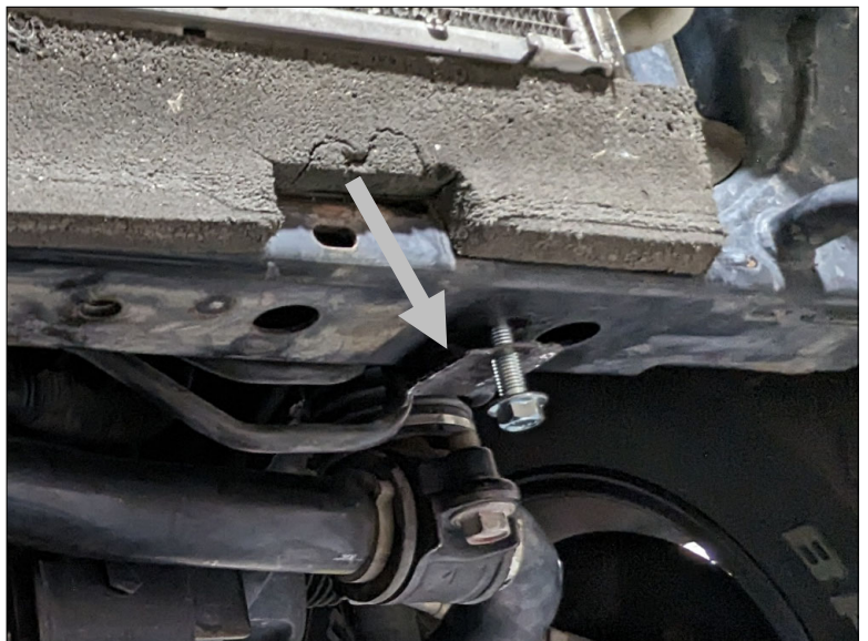
Step 7: One of the power steering line brackets flattened.
