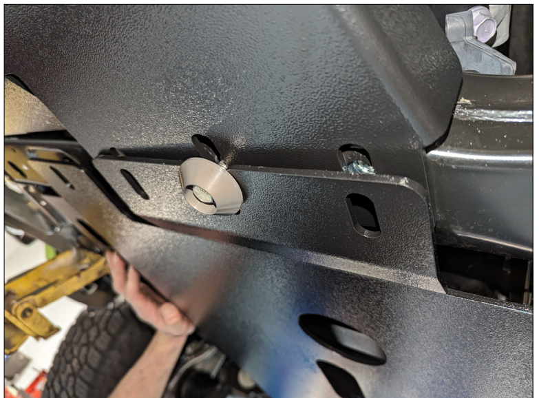
(Step 11) Transmission skid plate installed under Transfer Case Skid
