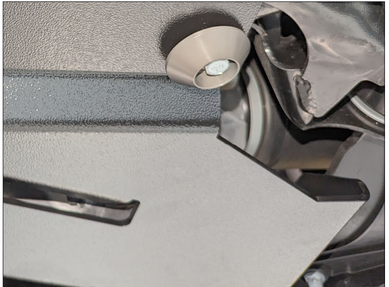
(Step 12) Bolt Protection Washer and M10 bolt installed on front of skid
