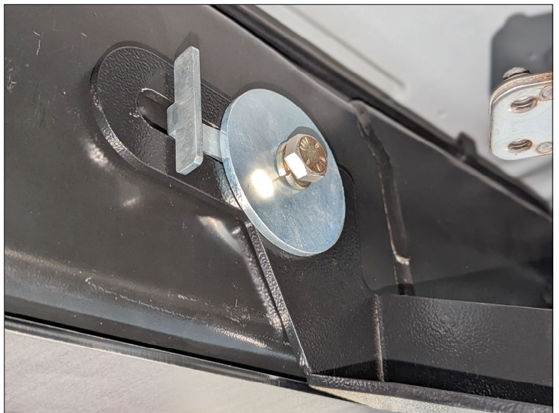
(Step 5 ) 3" washer is used to clamp the gusset to the frame
