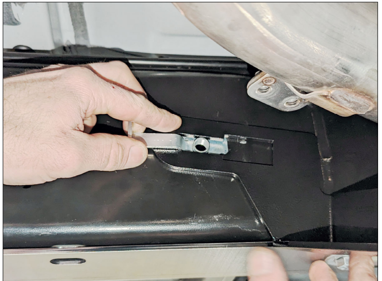
(Step 4 ) Transfer Case Gusset against frame with Frame Nut Plate
