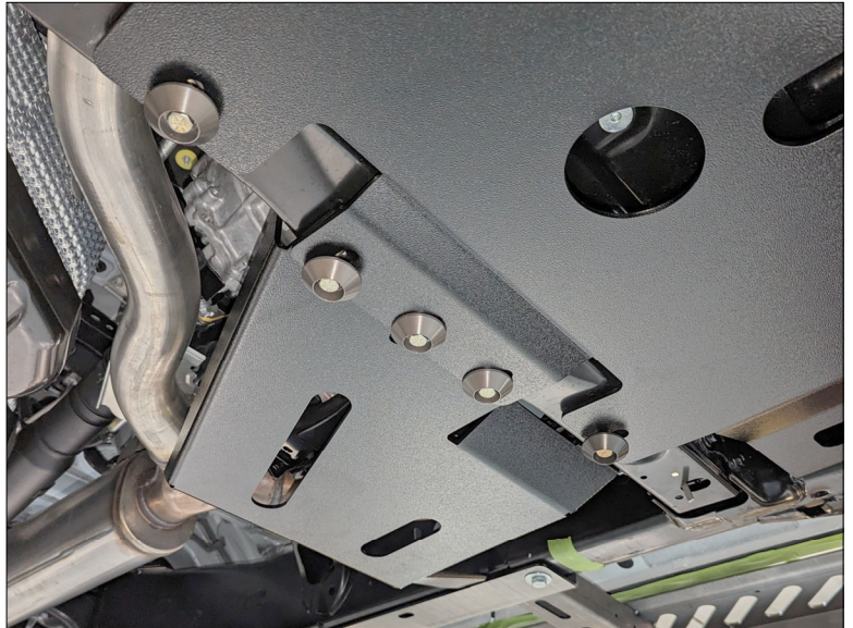
(Step 16) All hardware installed.
