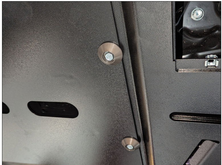
(Step 21 ) M10x 30 mm bolts with protection washers installed.
