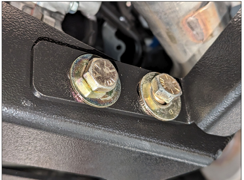
(Step 10) Transfer Case Gusset attached to Transfer Case Skid
