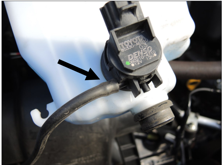
Cont. Plug outlet if reservoir has fluid in it. (Step 3)
