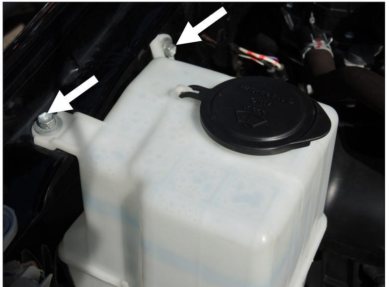
Remove the washer fluid reservoir. (Step 3)
