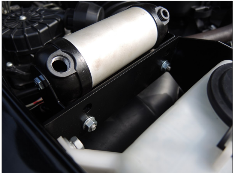
Install the manifold. (Step 13)
