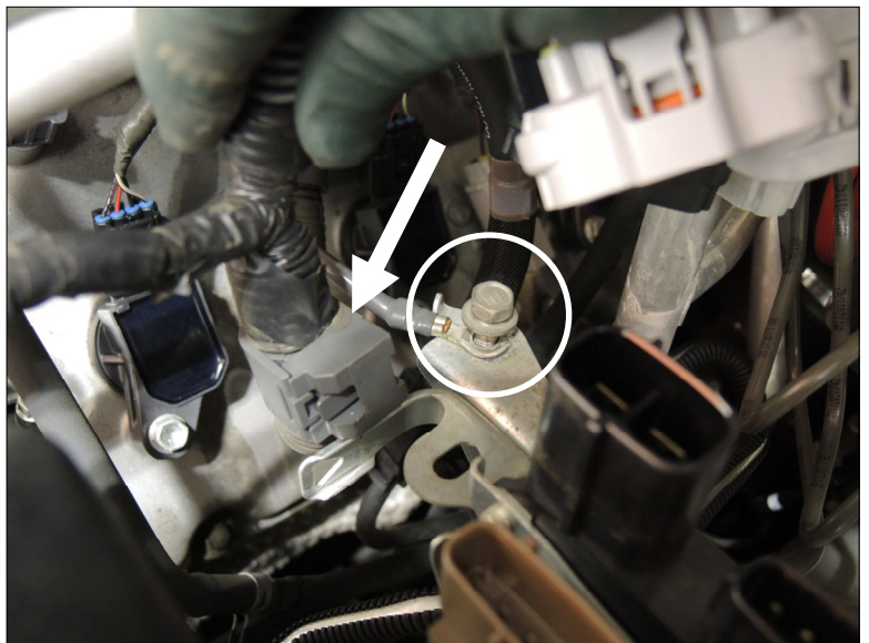
Unclip harness retainer Remove ground bolt. (Step 3)
