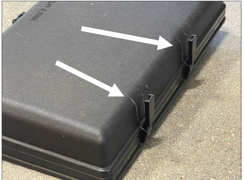
Trimming Fuse Box Lid Latches. (Step 14)
