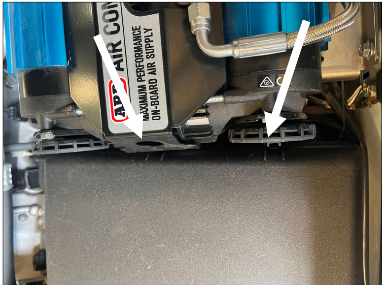
Clearance between filters and fuse box. (Step 15)
