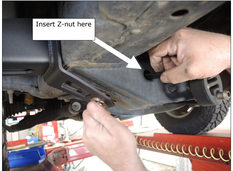
Step 5: Loosely Install Z-Nut and Bolt
