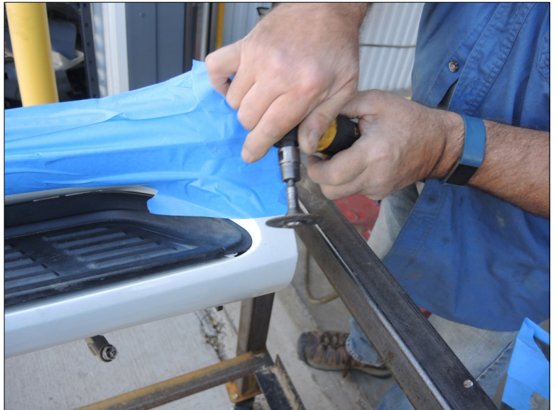
Mask the rocker cover with tape. (Step 4)
