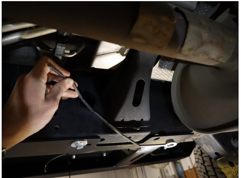
Shape a sticknut to fit the hole location. Secure with a bolt. (Step 18)
