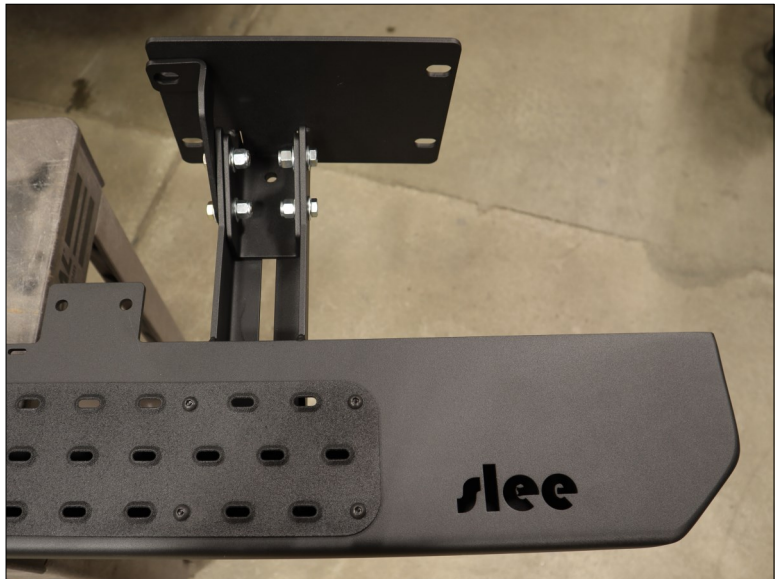
Loosely assemble the front leg and support. (Step 6)
