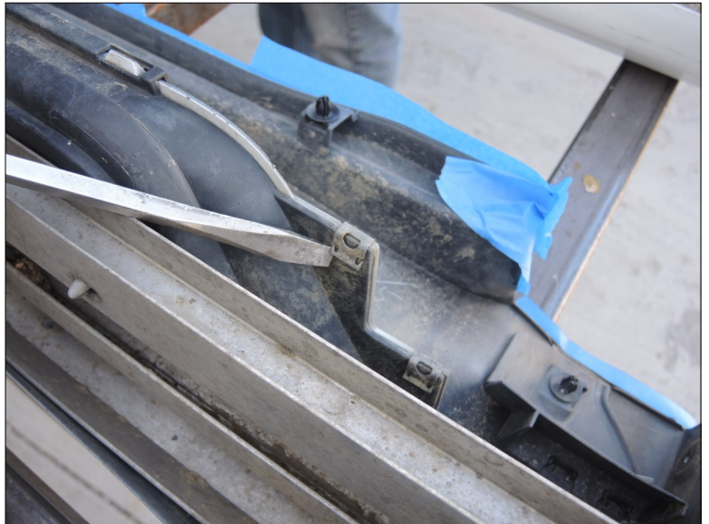
GX460: Separate the running board components. (Step 2)
