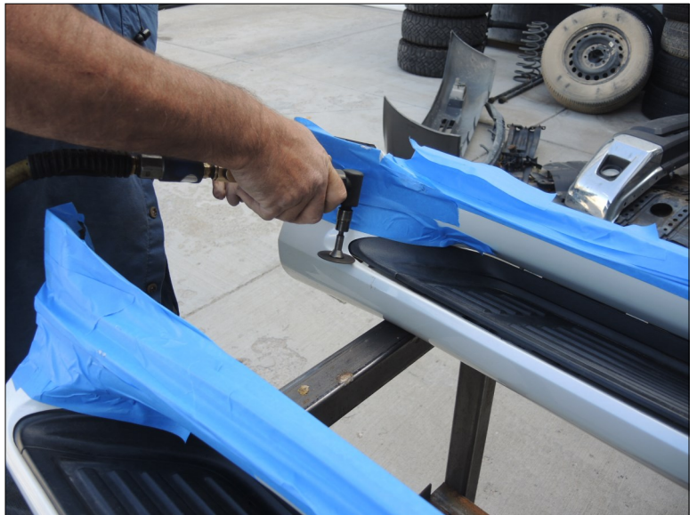
GX460: Separate the running board components. (Step 2)
