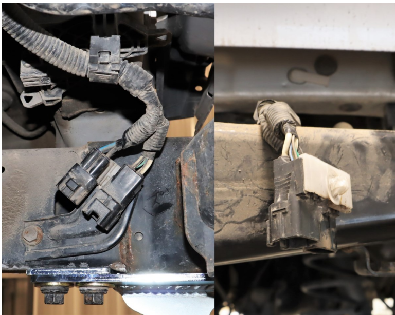
R&R the 7-pin wiring over the cross member (Step 14)
