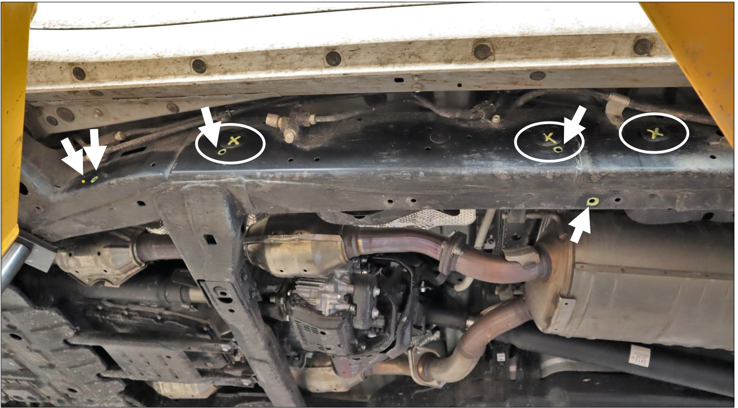
Install (5) rivet nuts into the driver side frame rail as indicated by arrows. Remove the (3) plastic frame plugs circled.
