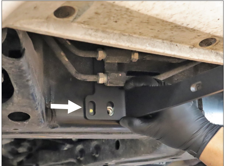
Mark driver side frame for hole. (Step 2)
