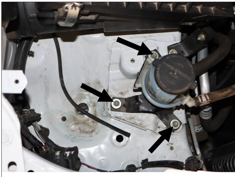
Remove the power steering reservoir bracket. (Step 2)
